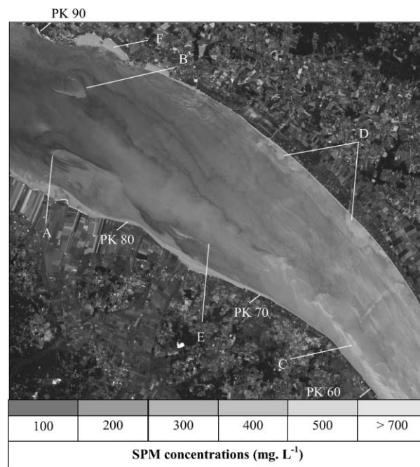
Fig. 17. SPOT-XS image (@CNES 14/07/96, 11:23 TU) of the downstream part of the Gironde estuary. The presented area is located in Fig. 1. The SPM concentrations were calculated from relationship presented in Fig. 10.
