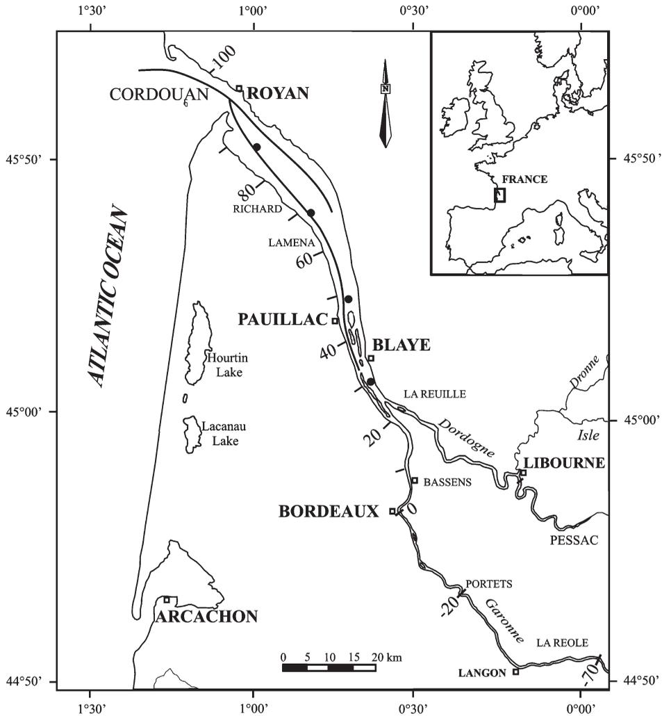
Figure 1. The Gironde estuary, located in south-west France. The lines represent the main navigation channels. Black circles locate the four stations of regular field measurements. The numbers indicate the distance (in km) from Bordeaux. These distances are called KP for kilometre points.
