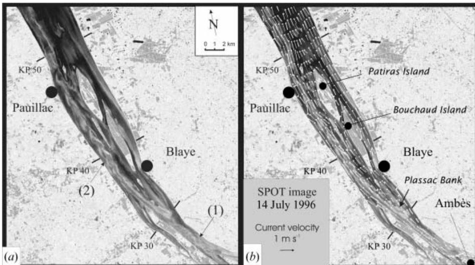
Figure 6. Example of detailed turbidity features observed on the SPOT image recorded on 14 July 1996. (a) Turbulent currents can be observed in the upstream part of the Gironde estuary. (b) Superposition of instantaneous current velocities calculated with the SAM-2D hydrodynamic model at the moment of satellite data acquisition.
