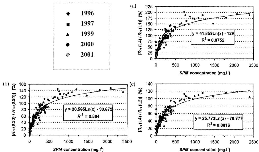
Fig. 7. Empirical relationships between reflectance ratios in (b) SPOT bands and in (a) and (c) Landsat bands and SPM, established from all field measurements carried out in the Gironde Estuary from 1996 to 2001. Plot of the logarithmic regression between 10 and  $2500 \text{ mg l}^{-1}$ .
